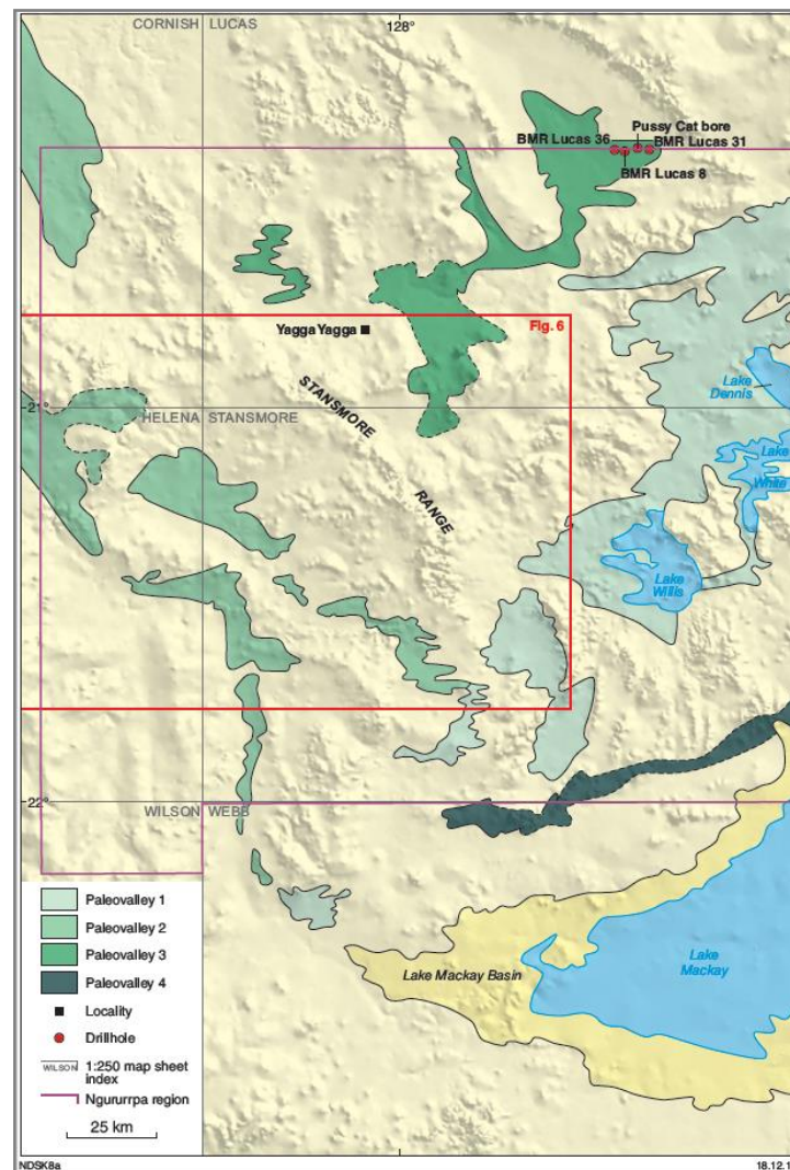
Figure 3: Distribution of four inset paleovalleys as part of an internal drainage network into Lake Mackay. The figure is draped on digital elevation model image. Three stratigraphic drillholes are shown intersecting Paleochannel 3 which reached the 91 m deep in drillhole BMR Lucas 36. Potable water was encountered between 14-16.5 m, below 4 m of calcrete and 10 m of sand in drillholes BMR Lucas 8 (paleochannel is 49 m deep) and BMR Lucas 31 (paleochannel is 88 m deep). Pussy Cat bore contained potable water between 14-16.5 m deep (Blake 1974).
