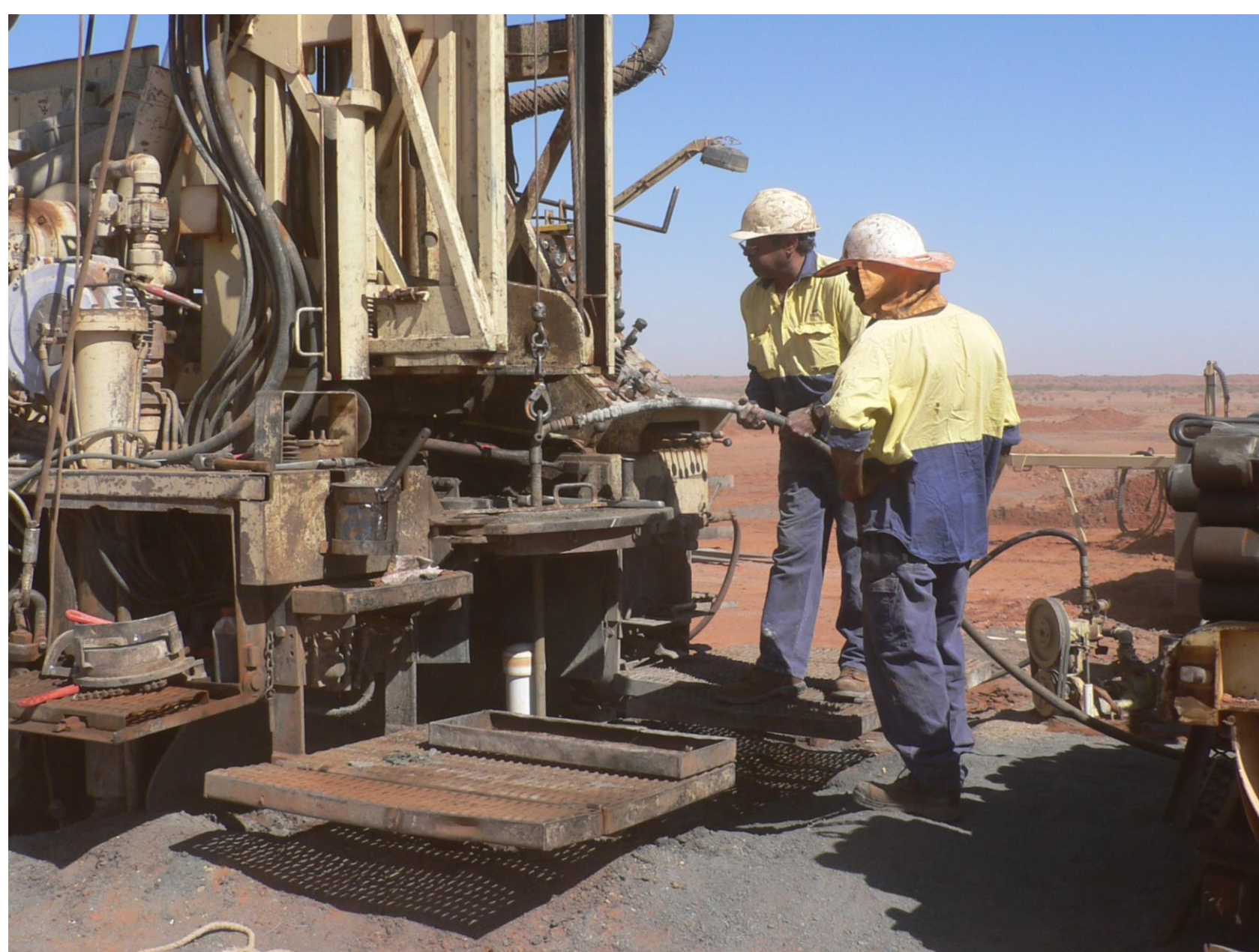
Targeted drilling of geophysical features to confirm hydrogeology
