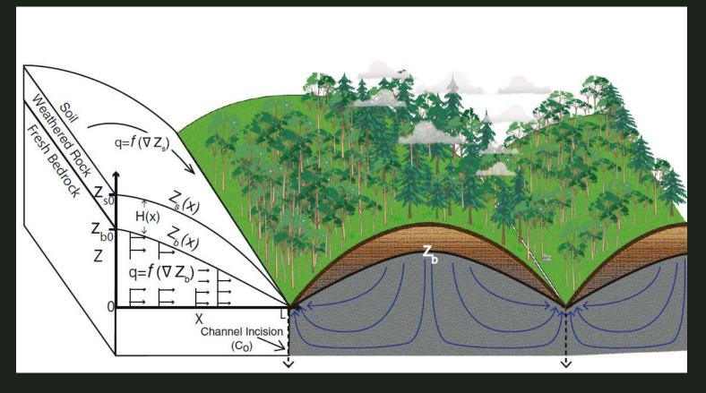
Conceptual model showing the elevation of fresh bedrock, Zb, under ridge and valley topography with a thin soil mantle overlying a weathered bedrock zone that extends to Zb. Channel incision, at the rate Co, drives hillslope erosion and drainage of fresh bedrock (flow paths illustrated with blue arrows). Source: Rempe and Dietrich, 2014
